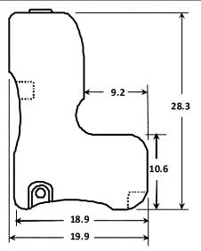
Figure 4(b). Side view of water dummy. All dimensions are in centimeters.
