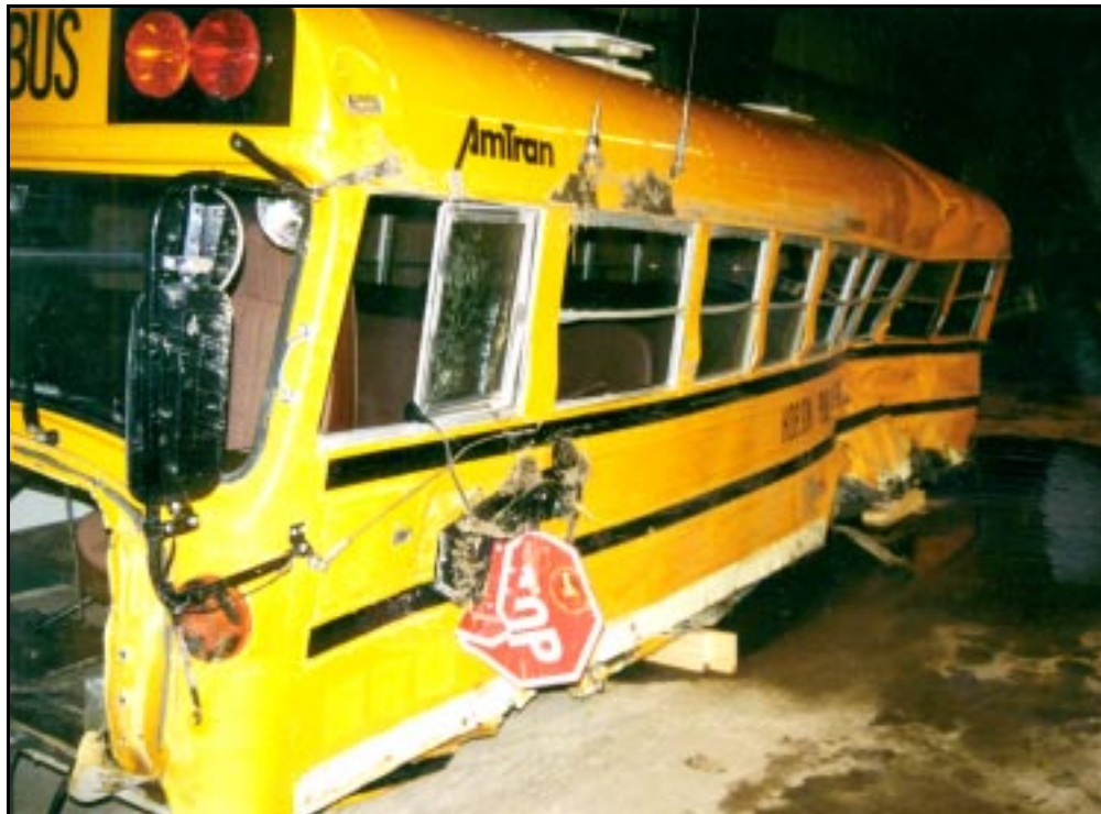
Figure 7. Buffalo school bus postaccident damage
