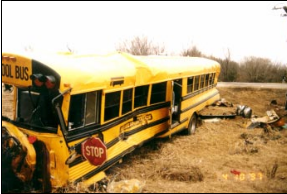
Figure 10. Monticello school bus postaccident damage
