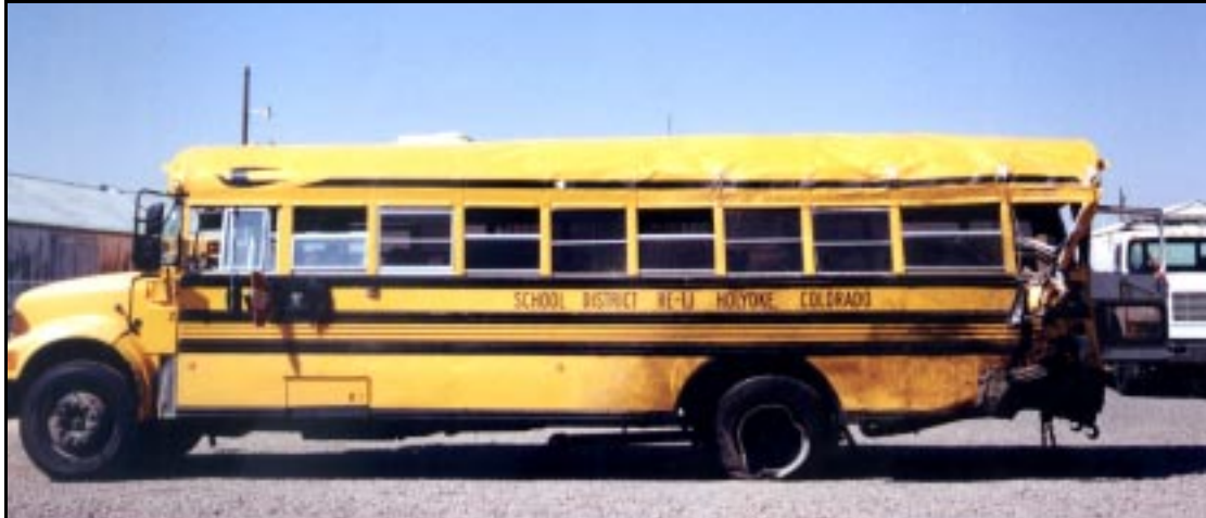
Figure 14. Holyoke school bus postaccident damage
