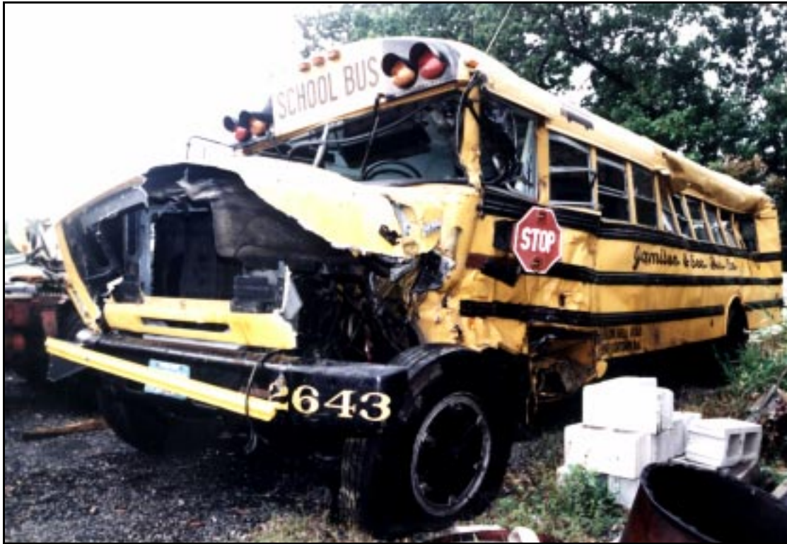
Figure 18. Holmdel school bus postaccident damage
