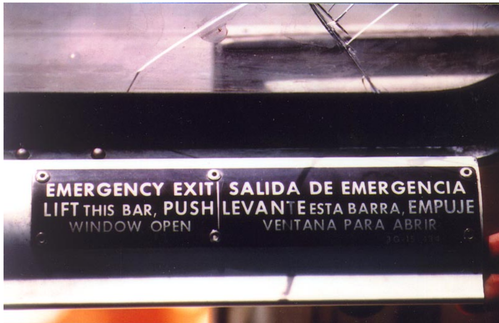
Figure 6. Instructions on motorcoach's emergency window release bar
