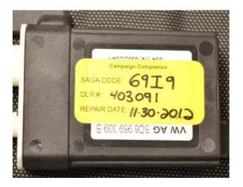
Fill out and affix Campaign Completion Label part number CAMP 010 000 to the PODS module prior to installation.
