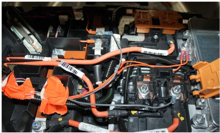
No. 021 Pre-Impact View of Ground Lead Attached
