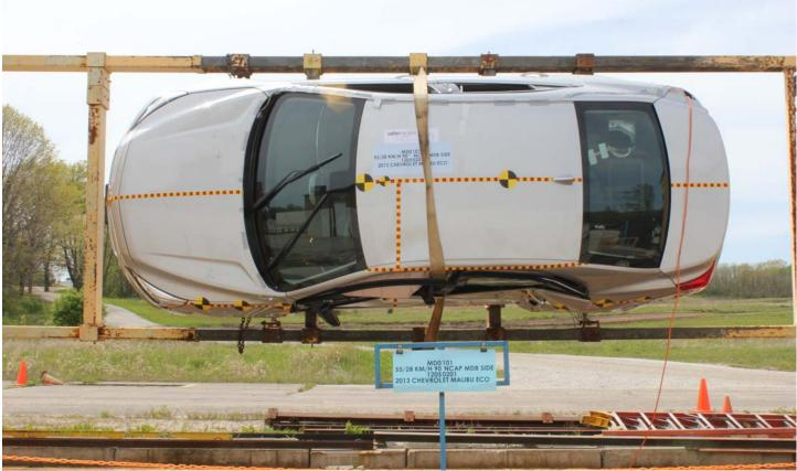
No. 030 FMVSS No. 305 Static Rollover at 270°
