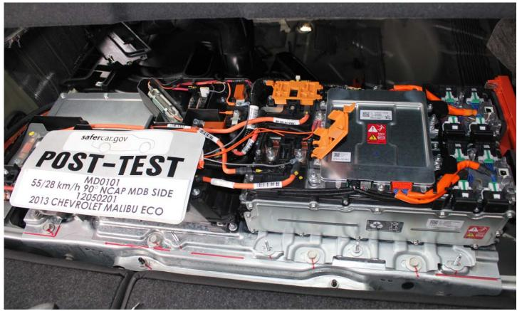
No. 015 Post-Impact View of Propulsion Battery Module(s)
