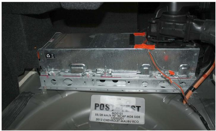
No. 011 Post-Impact Rear View of Propulsion Battery
