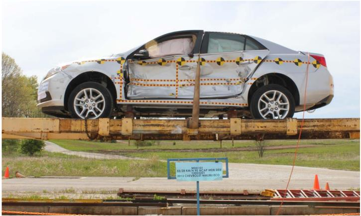
No. 031 FMVSS No. 305 Static Rollover at 360°
