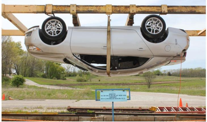
No. 029 FMVSS No. 305 Static Rollover at 180°
