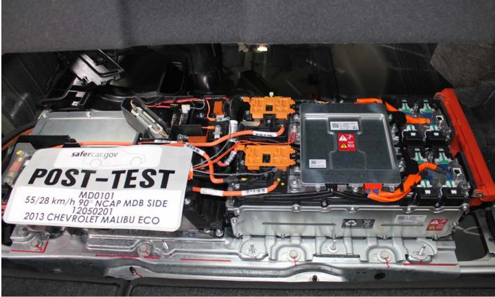
No. 010 Post-Impact Front View of Propulsion Battery
