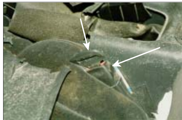
Figure 19: Close-up of case vehicle's engaged driver seat belt buckle and latch plate (case photo #39)
