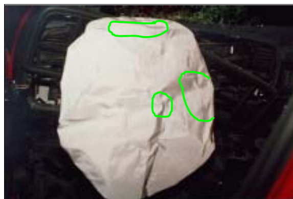
Figure 16: Case vehicle’s deployed driver air bag; Note: highlighted areas denote skin transfers (case photo #51)
