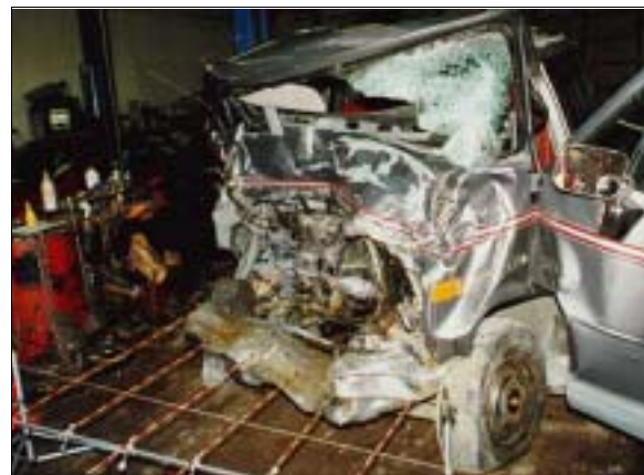
Figure 7: Vehicle #2's extensive, offset, frontal crush viewed from left of front with contour gauge present (case photo #65)
