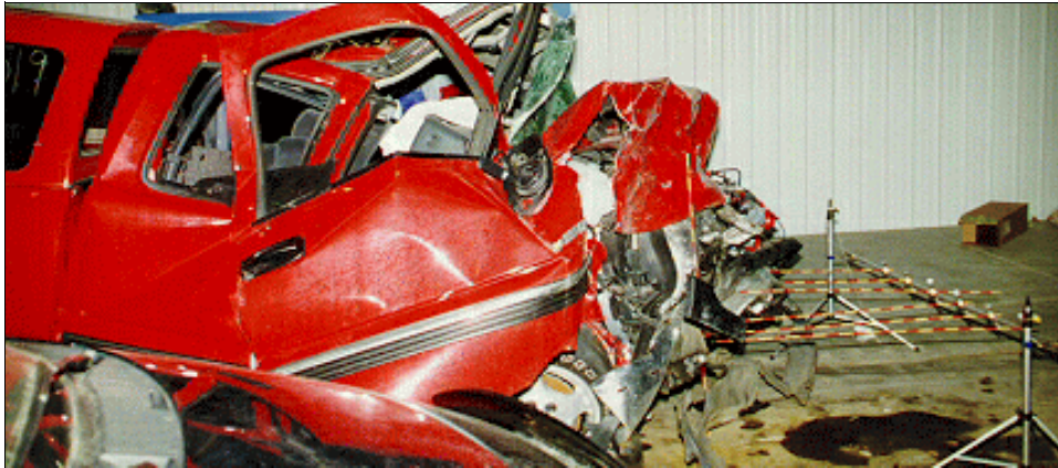
Figure 20: Right side view of extensive deformation to case vehicle's front (case photo #27)
