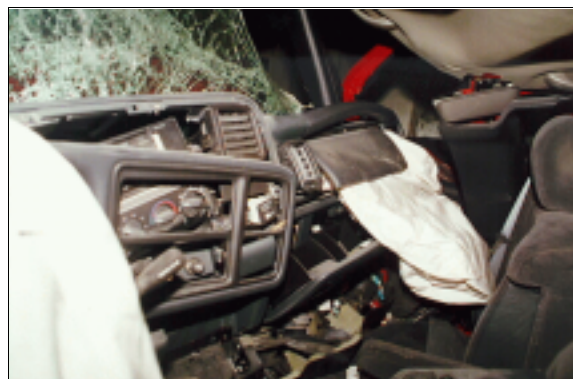
Figure 17: Case vehicle's deformed center instrument panel and front right seating area showing front right passenger air bag module's On/Off switch and module's cover flap and deployed air bag (case photo #59)
