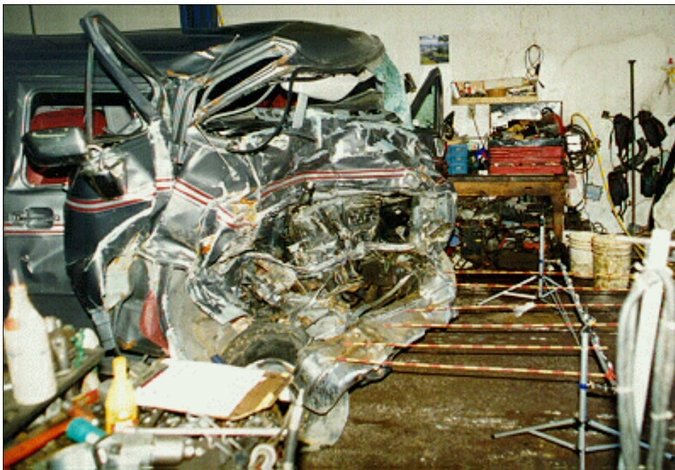
Figure 21: Vehicle #2's offset (toward right) frontal crush viewed along front reference line from right with contour gauge present (case photo #69)
