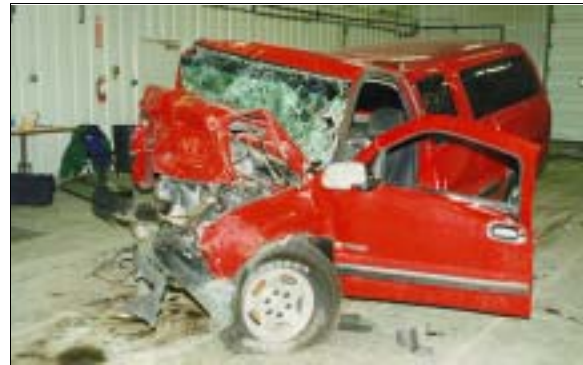
Figure 5: Extensive crush to case vehicle's front right portion viewed from left of front; Note: both "A"-pillars are deformed (case photo #14)
