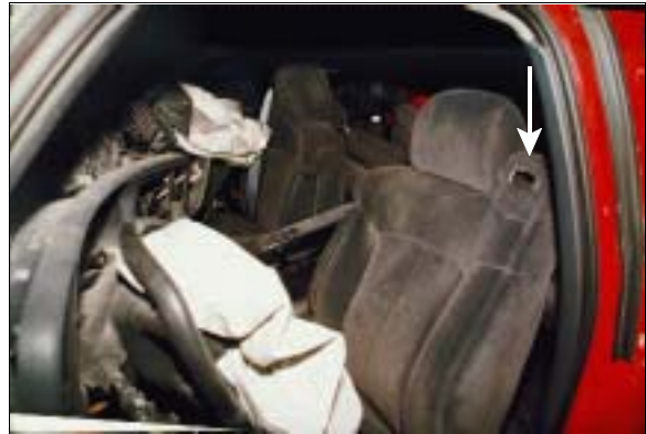
Figure 12: Case vehicle's driver seating area viewed from outside driver's door showing opening on seat back for driver's shoulder belt retractor; Note: intrusion to passenger area (case photo #42)
