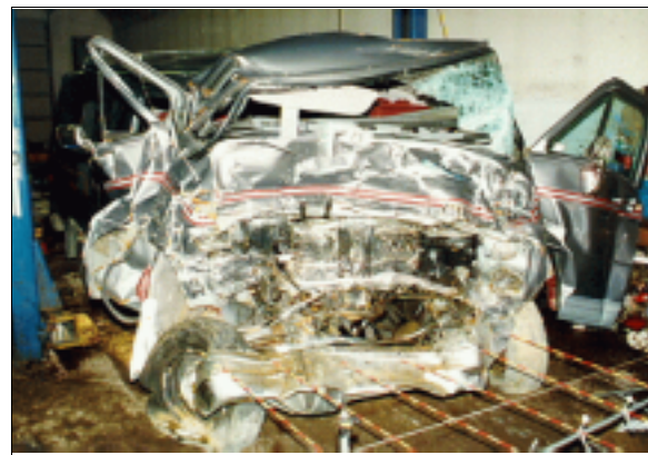
Figure 8: Vehicle #2's extensive, offset, frontal crush, with contour gauge present, viewed from right of front (case photo #70)
