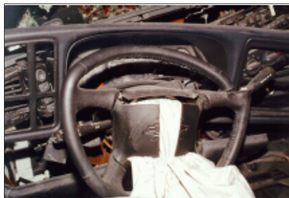
Figure 15: Case vehicle’s loaded and deformed steering wheel showing deployed driver air bag, “I”-configuration cover flaps, and cracked rim (case photo #49)
