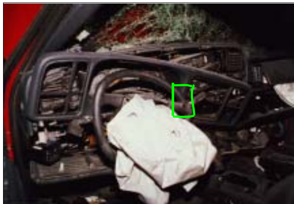
Figure 13: Case vehicle's driver seating area showing deployed driver air bag; Note: deformed and fractured steering wheel rim (case photo #46)
