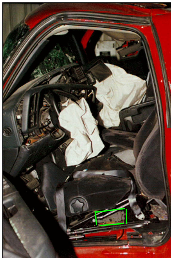
Figure 18: Case vehicle's front seating area viewed from outside driver's door showing intrusion to front right passenger seating area; Note: area highlighted under driver's seat is location of the S ensing and D iagnostic M odule (case photo #37)
