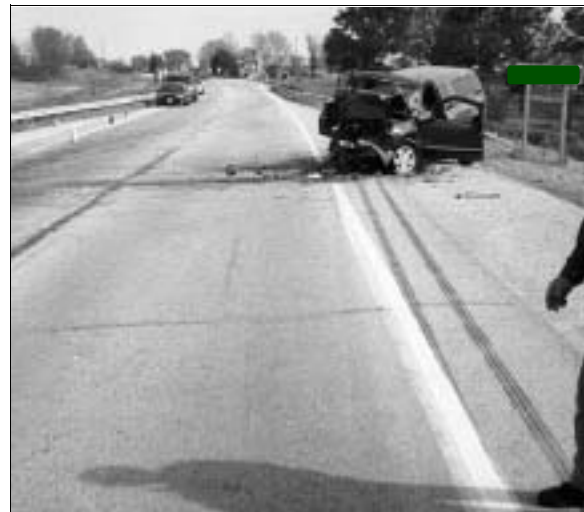
Figure 3: On scene northeastward view of case vehicle's final rest position on southeast shoulder and vehicle #2's straight line skid marks into impact near right (southeast) edge line; Note: case vehicle had been traversing a right-hand curve (case photo #04)
