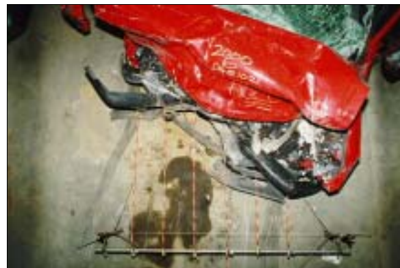
Figure 4: Overhead view of crush to case vehicle's front with contour gauge present showing offset (toward right) nature of crash (case photo #11)
