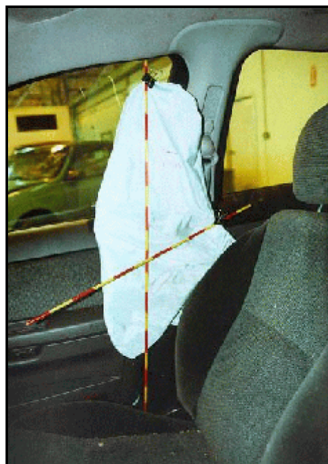
Figure 5. Deployed right front passenger's side air bag
