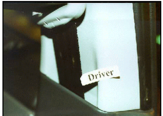
Figure 9. Load marks to driver's seat belt
