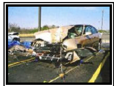
Figure 4. Frontal damage to the 2000 Chevrolet Impala.
