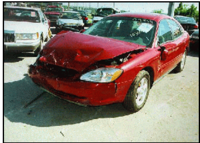
Figure 3. Left front quarter view, Ford Taurus. Shows second impact
