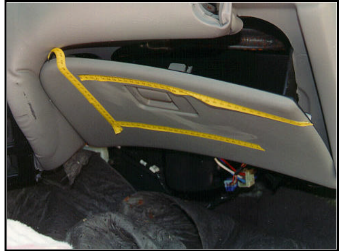
Figure 7. Scuff mark to glove box from contact with front right occupant's legs.
