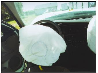
Figure 3. Case vehicle driver's air bag.
