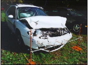
Figure 2. Frontal damage to case vehicle.
