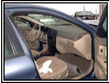
Figure 3. Interior view of the non-deployed frontal air bag modules.
