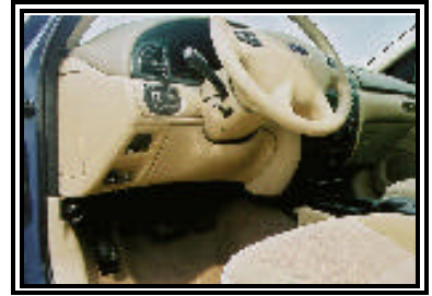
Figure 7. Steering wheel rim and knee bolster lacking contact evidence.
