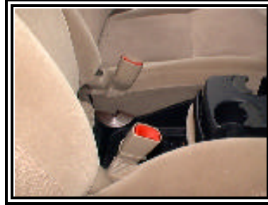
Figure 4. Non-fired front seat belt buckle pretensioners.
