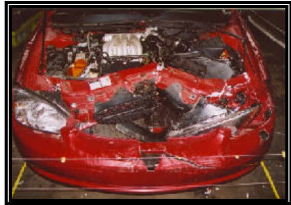
Figure 4: View of the damaged front plane.
