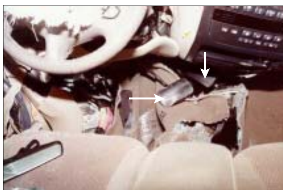
Figure 13: Case vehicle's adjustable brake (left) and accelerator (right) pedals; Note: severe toe and floor pan deformation and arrows locating pedals (case photo #40)
