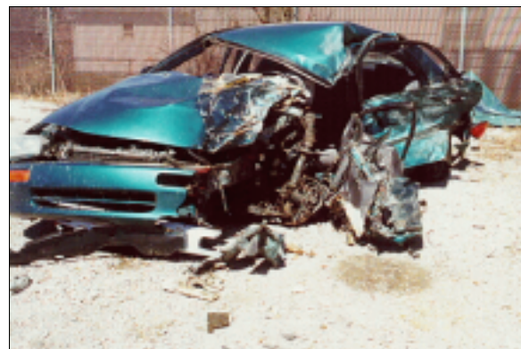
Figure 7: Mazda's frontal impact showing narrow end engagement and extensive damage and penetration to left side (case photo #62)
