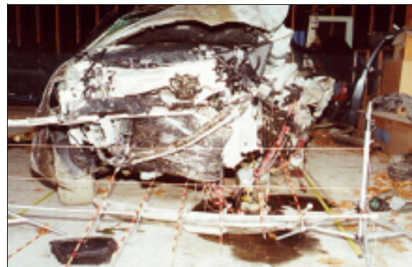
Figure 5: Case vehicle's front left damage with contour gauge present (case photo #14)
