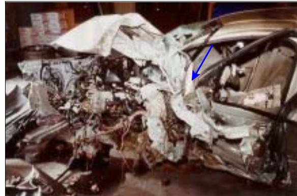
Figure 11: Damage extends down case vehicle's left side as a result of frontal impact; Note: arrow locates lower portion of left upper "A"-pillar (case photo #21)
