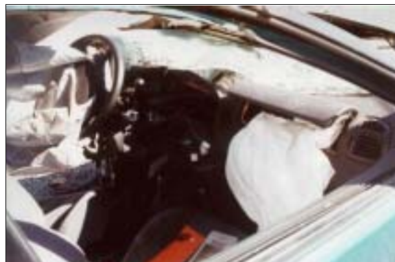
Figure 16: Mazda's deployed driver and front right passenger air bags viewed from right near "B"-pillar (case photo #85)
