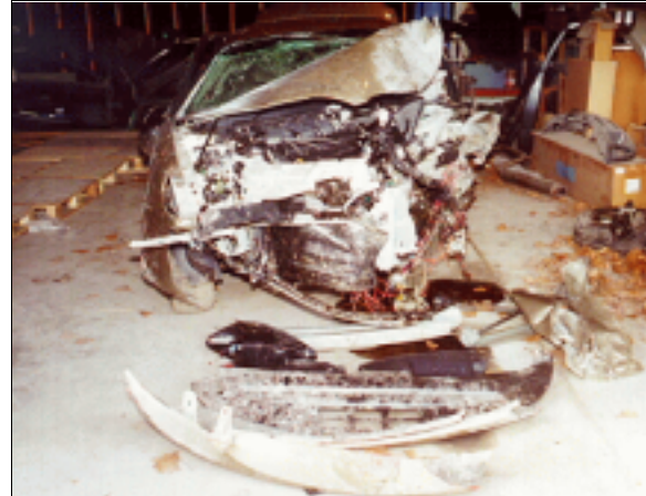
Figure 4: Case vehicle and damaged components; Note: direct frontal damage was primarily offset toward front left (case photo #13)
