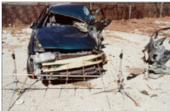
Figure 6: Mazda's narrow front left corner damage viewed from front; Note: front bumper fascia missing and driver's door toward right of photo (case photo #56)
