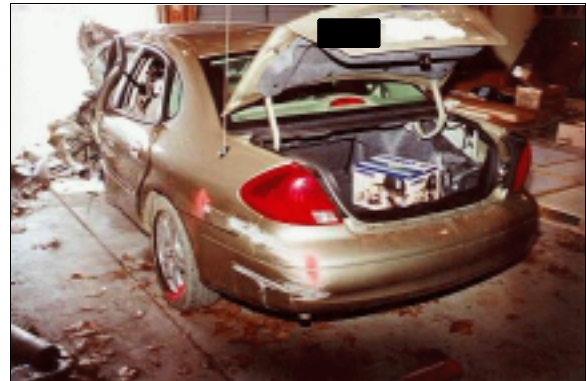
Figure 8: Case vehicle's back left sideswipe damage from contact with the median guardrail (case photo #24)
