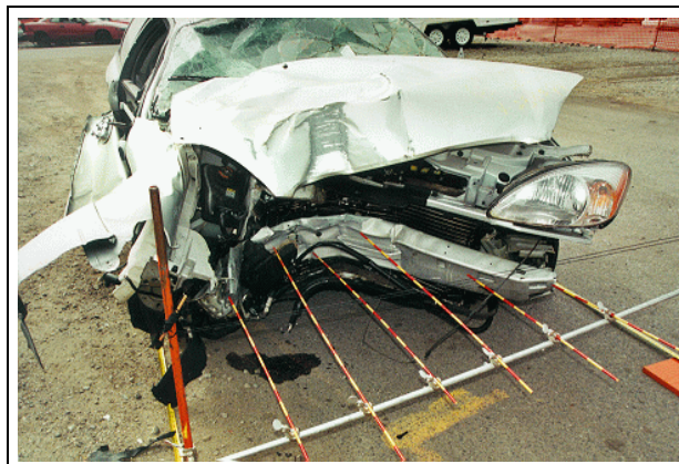
Figure 4. Exterior overlapping front damage to the case vehicle.
