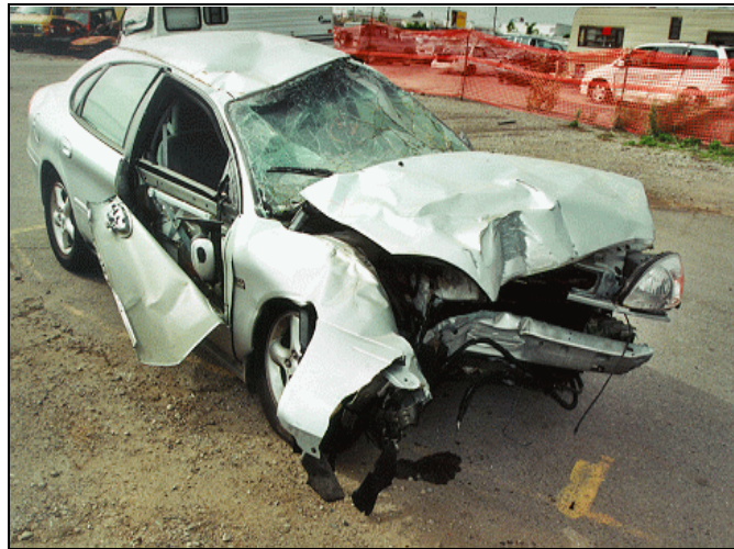
Figure 2. Rollover damage to case vehicle.
