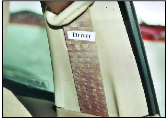
Figure 15. Seat belt loading marks on driver's belt
