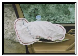
Figure 8: Front left side impact air bag.
