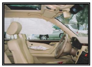
**Figure 11**: Right interior view of the head protection curtain.
