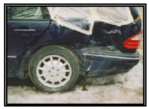
Figure 4: Close-up of the left rear quarterpanel damage.
