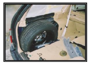
Figure 5: Damage to the spare tire compartment.
