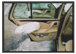
Figure 9: Rear left side impact air bag.
