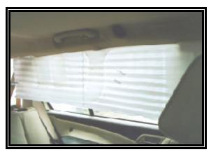
**Figure 12**: View of the rearward aspect of the head protection curtain.
