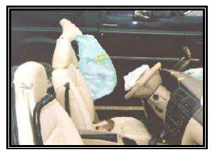
Figure 6: Left side impact air bag.
