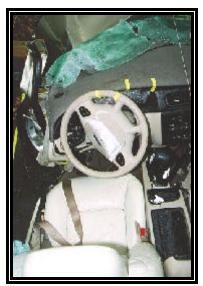
Figure 5: Interior intrusion.
