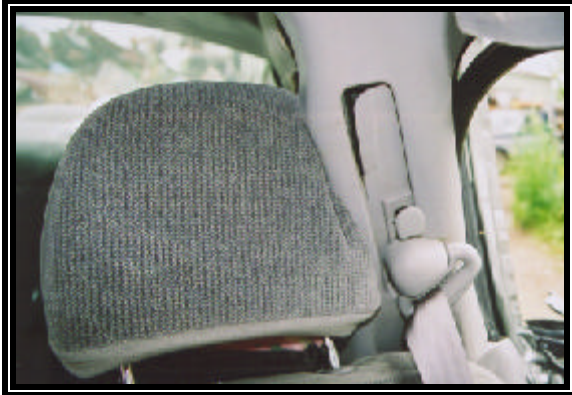
Figure 8: View of direct contact between the left B-pillar and driver's head restraint.
