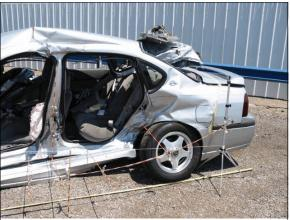
**Figure 7:** Damage to case vehicle's left side and specifically back left area from impact (1<sup>st</sup> event) with 2001 Accord; Note: doors removed for occupant extrication (case photo #18)
