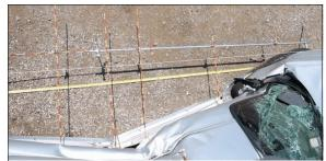
Figure 13: Overhead view of case vehicle's left side crush near left "B"-pillar and driver's door areas (case photo #23)
