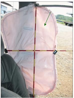
**Figure 22:** Inboard view of case vehicle's driver seat back-mounted side air bag showing internal tether stitching and faint occupant contact (arrow) on air bag's fabric (case photo #60)
