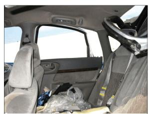
Figure 23: Case vehicle's back seating area and interior surface of intruded right rear door (case photo #76)
