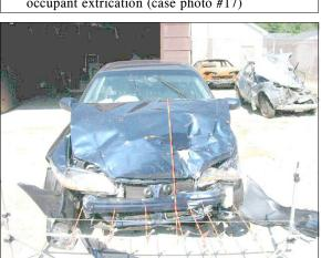
**Figure 8:** 2001 Accord's frontal damage from impact (1<sup>st</sup> event) with case vehicle's left side (case photo #83)
