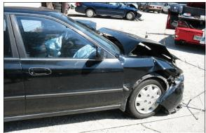
**Figure 26:** 1996 Accord's frontal damage viewed from back of right showing deployed frontal air bags and greater severity of crush at front right corner (case photo #110)
