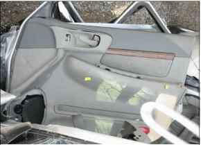
Figure 17: Interior surface of case vehicle's right front door showing suspected areas of occupant contact (case photo #51)
