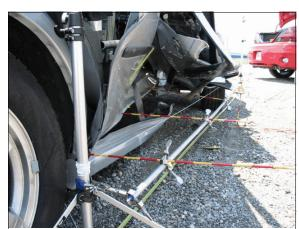
Figure 14: Sill level view from back right of case vehicle's right side crush (case photo #27)
