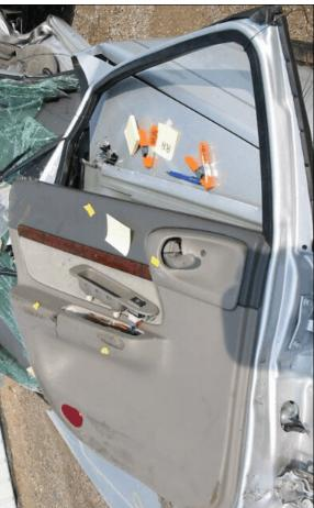
**Figure 16:** Interior surface of case vehicle's left rear door showing intrusion damage and evidence of possible occupant contacts (case photo #78)
