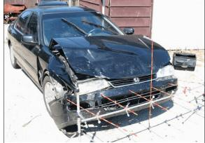
Figure 27: 1996 Accord's frontal damage viewed from right of front with contour gauge present (case photo #111)
