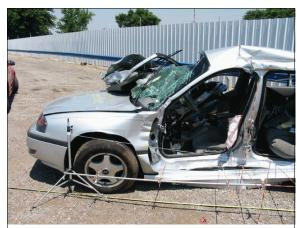
**Figure 6:** Damage to case vehicle's left side and specifically driver's area from impact (1<sup>st</sup> event) with 2001 Accord; Note: doors removed for occupant extrication (case photo #17)
