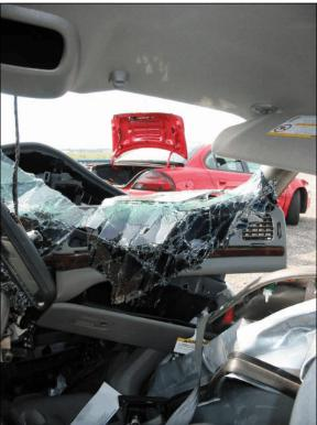
Figure 30: Case vehicle's front right passenger seating area showing lateral and vertical intrusion to right instrument panel (case photo #50)
