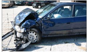
Figure 24: 2001 Accord's frontal damage viewed from left; Note: severity of crush and deployed frontal air bags (case photo #88)
