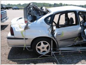
**Figure 10:** Damage to case vehicle's right side, rear half, from impact (2<sup>nd</sup> event) with 1996 Accord; Note: distortion to right rear door and intrusion at sill level near "B"-pillar (case photo #28)
