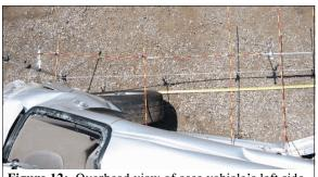
Figure 12: Overhead view of case vehicle's left side crush near left rear door area (case photo #22)
