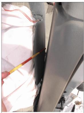
**Figure 21:** Cover flap from case vehicle's driver seat back-mounted side impact air bag (case photo #65)
