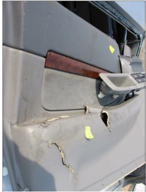
Figure 15: Interior surface of case vehicle's left front door showing driver's contacts and damage from intrusion (case photo #81)
