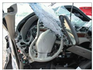
**Figure 20:** Case vehicle's steering wheel rim and left instrument panel deformed by lateral intrusion into driver's door (case photo #47)
