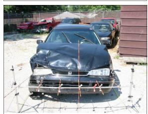
Figure 9: 1996 Accord's frontal damage from impact (2<sup>nd</sup> event) with case vehicle's right side (case photo #98)
