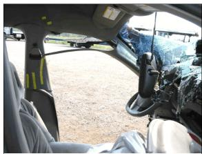
Figure 18: Case vehicle's front seating area showing suspected occupant contacts to left roof side rail and left "B"-pillar areas (case photo #54)
