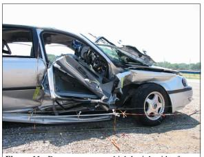
**Figure 11:** Damage to case vehicle's right side, front half, from impact (2<sup>nd</sup> event) with 1996 Accord (case photo #29)
