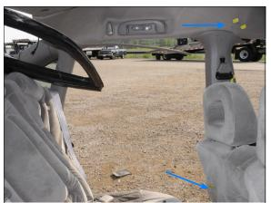
Figure 19: Case vehicle's back seating area showing contact evidence on left roof side rail near left "B"-pillar and back left of driver's seat back; Note: removed left side doors (case photo #77)
