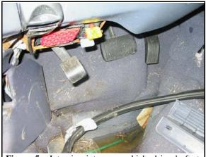
Figure 5: Intrusion into case vehicle driver's foot well area (case photo #37)
