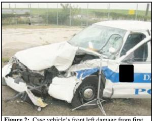
Figure 2: Case vehicle's front left damage from first (most severe) impact; note wheel damage from curb impact, front right wheel also damaged (case photo #18)
