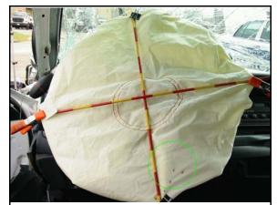
Figure 6: Front of case vehicle driver's air bag (top of bag at left in this photo); note blood drops (highlighted) in the 9 o'clock region (case photo #48)
