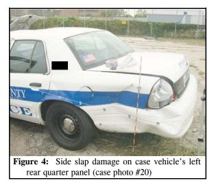
this secondary impact, based on the measured crush profiles of both vehicles. The results indicated Total, Longitudinal and Lateral DeltaVs, respectively: 8.0 km.p.h. [5.0 m.p.h.], 0 km.p.h. [0 m.p.h.] and +8.0 km.p.h. [+5.0 m.p.h.]. These results appear reasonable. The case vehicle also sustained left and right front wheel impacts as it mounted the curb, with CDCs 12-FLWN-3 and 12-FRWN-3.
