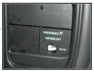
Figure 7. Front right passenger air bag cut off switch
