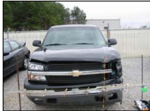
Figure 5. Chevrolet's crush profile.
