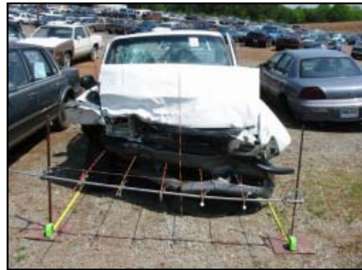
Figure 7. Frontal damage to the 1994 Mazda B2300.
