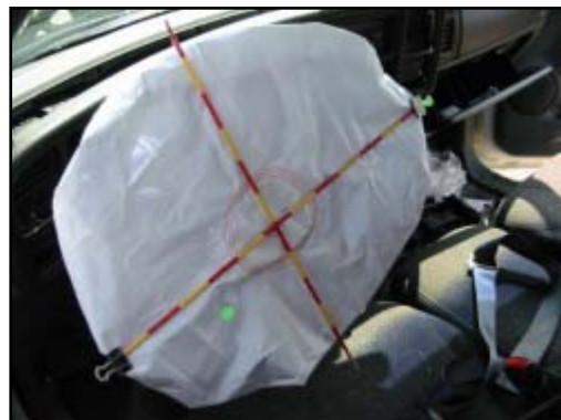
Figure 12. Deployed driver's air bag.
