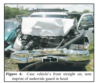
were crushed rearward against the engine block. The hood was buckled nearly double and the trailing edge of the hood was forced rearward, causing heavy cracking of the windshield glazing across the entire width. There was no other glazing damage. The leading edge of the right fender
