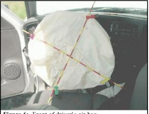
Figure 6: Front of driver's air bag
