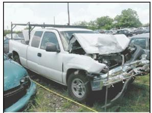
Figure 3: Case vehicle's front and right side; note, front frame rails shifted upward
