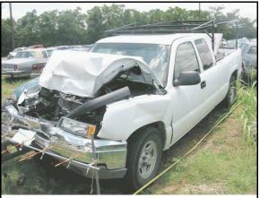
Figure 2: Case vehicle's front and left side; note, direct contact heavier on right
