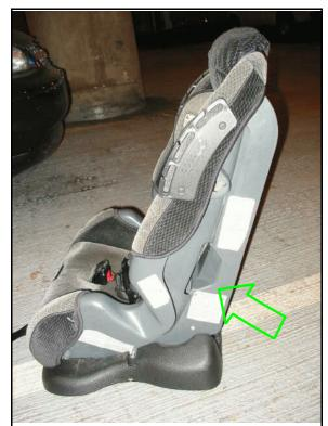
**Figure 9:** Left side of CSS; seat was secured by vehicle's lap-and-shoulder belt in manufacturer's designated slot (arrow) (case photo #56)
