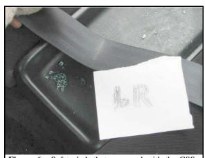
**Figure 6:** Safety belt that was used with the CSS, showing loading marks (case photo #47)
