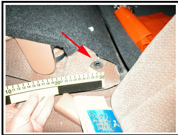
Figure 9. Bottom hinge failure
