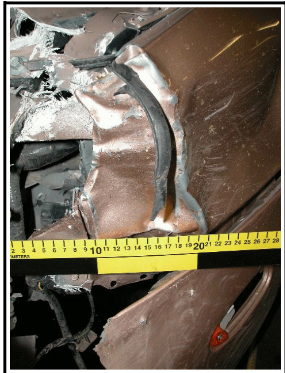
Figure 7. Close up of damage from initial impact
