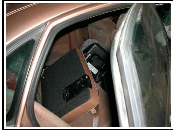
Figure 8. Rear seat back failure
