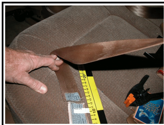
Figure 23. Rear left seat belt—shows loading and point where it was cut off
