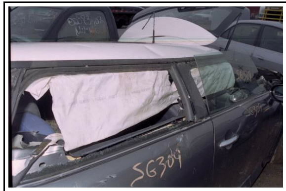
Figure 9. Exterior view, left side air curtain (roof had been cut off and was put back onto vehicle backwards)
