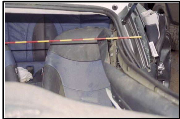
Figure 13. Left side intrusion
