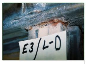
**Figure 18.** Cracked weld at the left D-pillar of Exemplar Bus No. 3.
