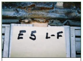
**Figure 22.** Cracked weld at left F-pillar of Exemplar Bus No. 5.
