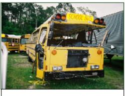
**Figure 5.** Front right view of the bus with the roof repositioned.
