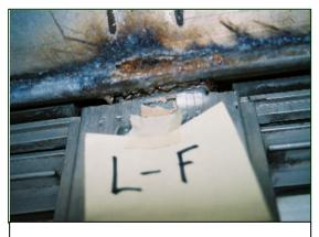
Figure 9. Crack at left F-pillar weld.
