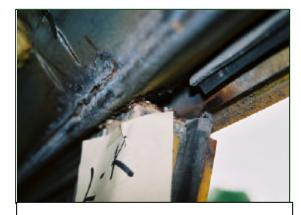
**Figure 10.** Tear and cracked welds at the left K-pillar
