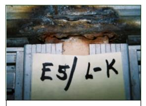
**Figure 23.** Complete crack of weld at left K-pillar of Exemplar Bus No. 5.
