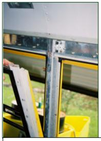
**Figure 15.** Continuous roof bow/pillar in the 1998 Carpenter bus.
