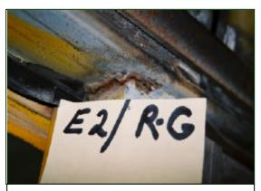
**Figure 17.** Cracked weld at the right G-pillar of Exemplar Bus No. 2.
