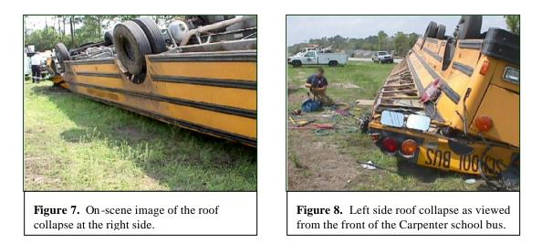
The right side doors were displaced laterally left by the roof deflection. The lower right B-pillar separated from the sill, resulting in body panel separation. Six screw fasteners pulled through the sheet metal resulting in the separation of the lower panel.
