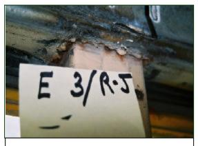
**Figure 19.** Cracked weld a the right J-pillar of Exemplar Bus No. 3.
