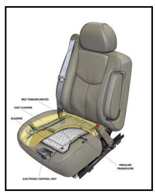
**Figure 4**. Front right Passenger Sensing System
