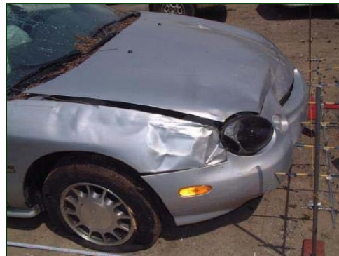
Figure 4. Lateral view depicting the depth of frontal crush.
