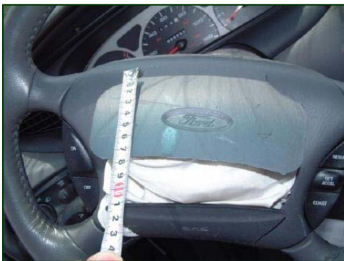
Figure 10. Driver air bag module cover flaps.
