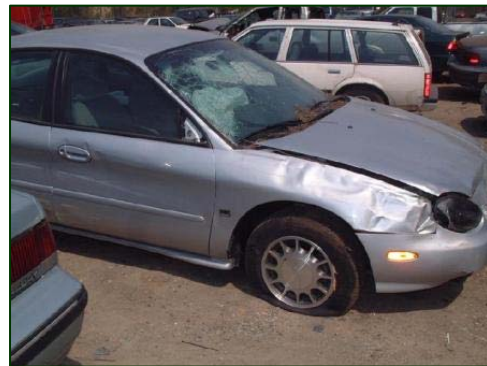
Figure 8. Right front fender sideswipe damage.
