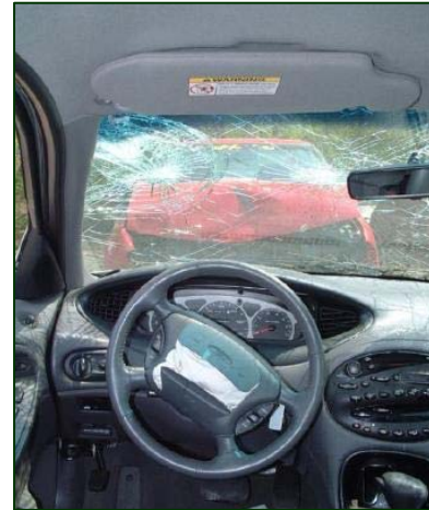
Figure 12. Initial trajectory of the unrestrained driver.
