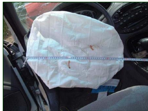
Figure 11. Deployed driver's redesigned frontal air bag.
