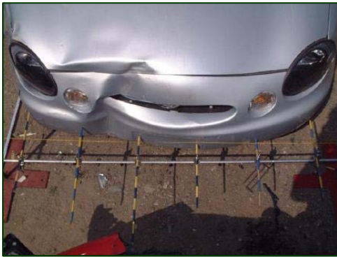
Figure 7. Overhead view of the frontal crush depth.
