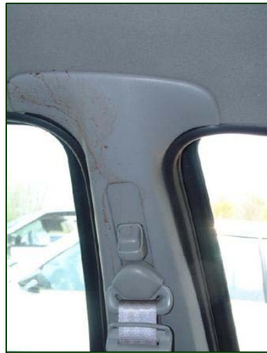
Figure 14. Head strike to the upper left B-pillar.
