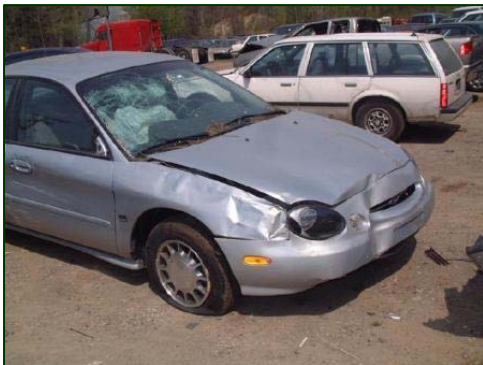
Figure 3. Frontal and right side damage to the Taurus.
