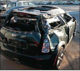
**Figure 7**. Right rear view showing rollover damage and contact to other vehicle
