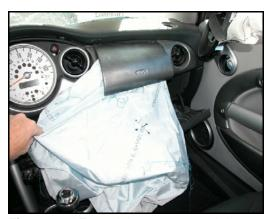
Figure 12. Front right passenger air bag
