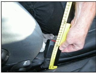
**Figure 13**. Driver's buckle mounted seat belt pretensioner
