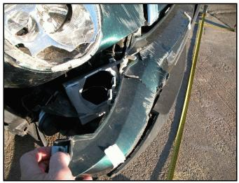
Figure 5. Close up view of reinforcement bar movement
