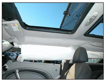
**Figure 20**. Front right seat area—shows contacted side air curtain
