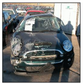
**Figure 8**. Rock damage to right bumper corner
