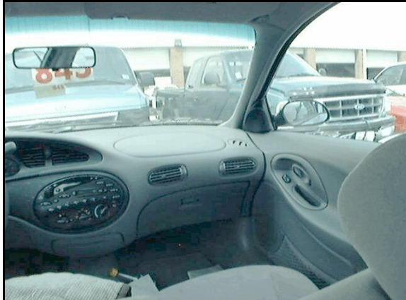
Figure 5: EXEMPLAR vehicle, showing non-deployed front right passenger's air bag module NOT THE CASE VEHICLE (case photo #13)
