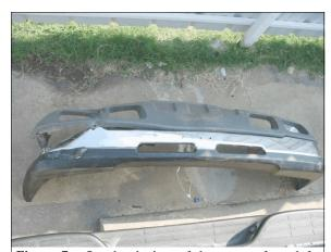
Figure 7: Overhead view of damage to front left portion of case vehicle's front bumper fascia and jounce bumper (case photo #25)
