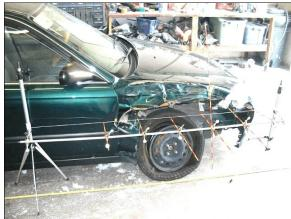
**Figure 13:** Damage to Honda's right fender and right front wheel assembly with contour gauge present above sill level (case photo #44)
