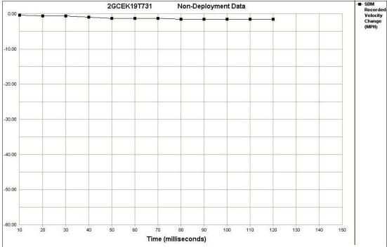
Figure 17: The case vehicle sustained a velocity change of approximately 2.6 km.p.h. (1.6 m.p.h.) during the first 120 milliseconds after the crash was detected
