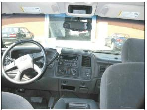
Figure 10: Case vehicle's driver seating area and center instrument panel showing non-deployed driver air bag and no apparent evidence of occupant contact to steering wheel, center instrument panel, or greenhouse areas (case photo #29)
