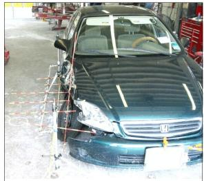
**Figure 4:** Elevated reference line view of Honda's right side damage with contour gauge present above sill level (case photo #37)
