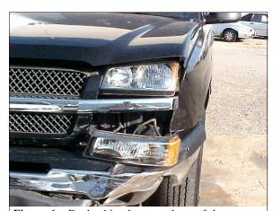
Figure 6: Dealership close-up photo of damage to case vehicle's front left bumper and left headlight and turn signal assemblies (case photo #18)
