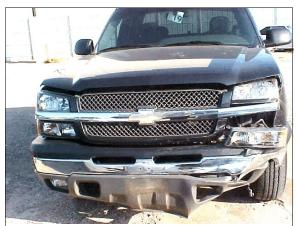
**Figure 3:** Dealership photo of case vehicle's frontal damage; Note: left side of jounce bumper driven rightward and rearward (case photo #15)
