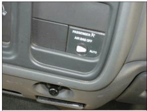
Figure 11: Close-up of case vehicle's center instrument panel showing front right air bag control switch in "auto" position (case photo #30)
