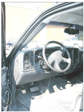
Figure 9: Case vehicle's driver seating area showing non-deployed driver air bag and foot well and no apparent evidence of occupant contact to left instrument panel, driver's knee bolster, and left "A"-pillar, windshield glazing, or sun visor (case photo #27)
