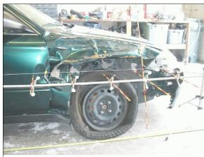
Figure 14: Close-up of damage to Honda's right fender, right front door, and right front wheel assembly (case photo #45)
