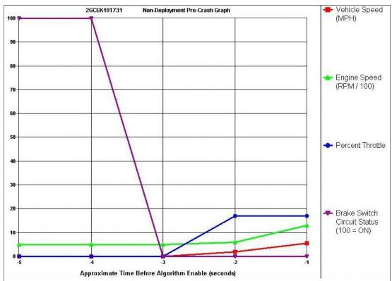
**Figure 16:** Case vehicle's pre-crash speed and brake switch circuit status showing that the vehicle had accelerated to approximately 10 km.p.h. (6 m.p.h.) and that the brake switch had been deactivated approximately 3 seconds prior to algorithm enable.
