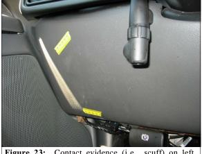
**Figure 23:** Contact evidence (i.e., scuff) on left portion of case vehicle's driver knee bolster (case photo #46a)
