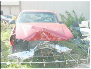
Figure 19: Case vehicle's frontal damage from impact with large tree; Note: contour gauge set at bumper level (case photo #29)
