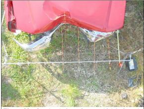
Figure 20: Overhead view of case vehicle's frontal damage from tree impact with contour gauge set at bumper level (case photo #41)
