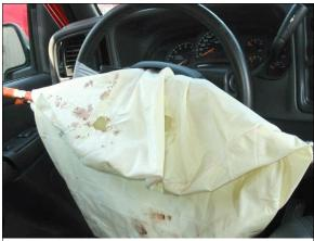
Figure 25: Case vehicle's deployed driver air bag showing blood stains on left upper quadrant of bag's back surface (case photo #51)
