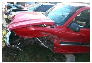
Figure 7: Case vehicle's left front damage from impact with Peterbilt's logging trailer; Note: left front wheel assembly sheared off by trailer (case photo #33)
