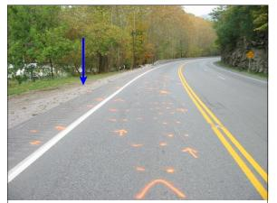
**Figure 5:** Peterbilt's estimated area of impact with Ford in western travel lane (i.e., foreground), estimated area of impact with case vehicle on northern shoulder (i.e., arrow), and subsequent easterly travel path toward impact with guardrail (case photo #03)
