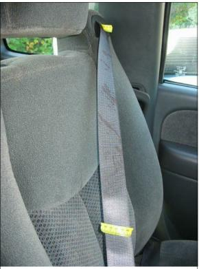
Figure 26: Blood stains on outward surface of shoulder portion of case vehicle's driver safety belt (case photo #55)
