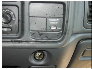
Figure 8: Case vehicle's front right passenger air bag cutoff switch set to "Auto" (case photo #48)
