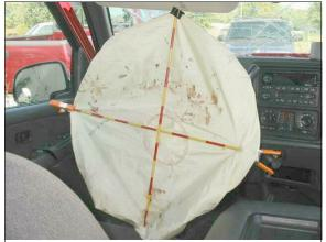
**Figure 24:** Case vehicle's deployed driver air bag showing copious blood evidence over three quadrants of the bag's front surface (case photo #50)
