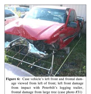
*Crash:* According to the case vehicle's driver, as the Peterbilt was tipping over onto its left side (**Figure 5**), an unknown portion of the Peterbilt collided with the left frontal portion of the Ford, shearing off the top portion of the Ford pickup's cab. The Peterbilt's semitrailer began to rotate clockwise (i.e., in a jackknifing fashion) after impacting the Ford. The Peterbilt continued forward in its easterly travel path, but it veered off the roadway onto the northern roadside.
