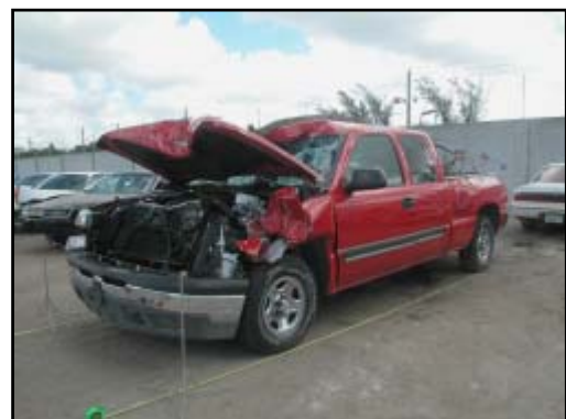
Figure 4. Frontal damage to the Silverado
