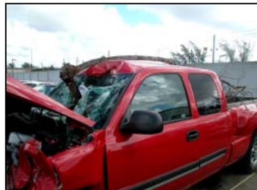
Figure 6. View of windshield header damage and tree limb
