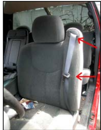
Figure 9. View of driver's safety belt highlighting webbing crease and scuff mark
