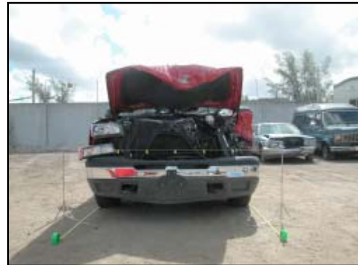
Figure 5. Frontal view of the damaged Silverado
