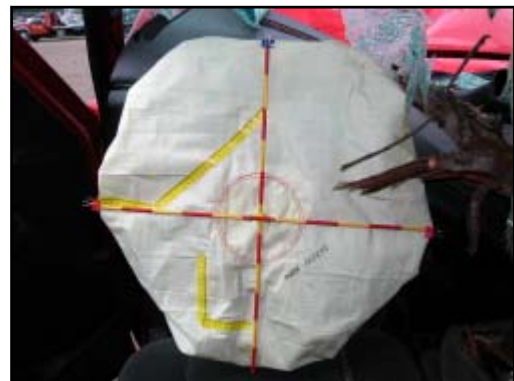
Figure 10. Deployed driver's air bag
