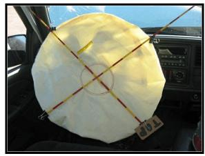
Figure 9. Face of driver's air bag
