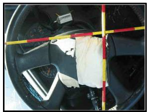
Figure 10. Driver's air bag module cover
