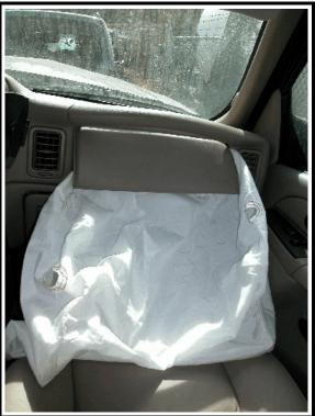
Figure 8. Front right passenger's air bag
