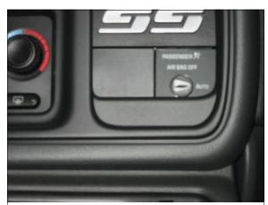
**Figure 6:** Front right air bag suppression switch, found in the "Auto" position (case photo #27)
