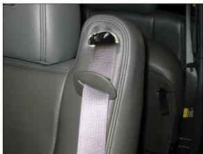
**Figure 13:** Driver's shoulder belt guide pulled out of the seat (case photo #33)
