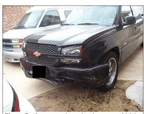
Figure 7: Insurance photo showing case vehicle's front damage from impact with Honda (case photo #12a)
