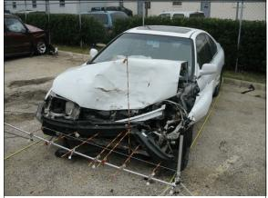
Figure 14: Damage to front of Honda from impact with case vehicle, each stripe on rods is 5 cm (2 in) (case photo #35)
