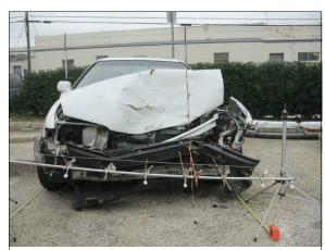
Figure 4: Honda's front damage from impact with the case vehicle (case photo #34)
