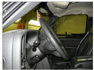
Figure 9: Left side view of steering wheel and steering column showing lack of deformation (case photo #18)
