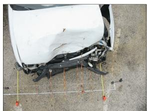
**Figure 15:** Top view of Honda's front crush (case photo #40)
