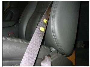
Figure 12: Ripple in driver's shoulder belt webbing between the pieces of yellow tape (case photo #30)
