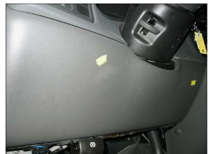
Figure 8: Yellow tape shows occupant contact scuffs on driver's knee bolster (case photo #22)
