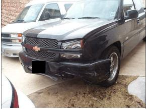
Figure 3: Insurance photo of case vehicle's front damage from impact with Honda (case photo #12a)
