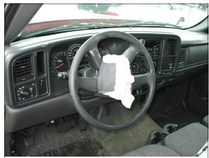
Figure 15: Case vehicle's deployed driver air bag and left and center instrument panel areas; Note: no obvious evidence of contact to instrument panel areas (case photo #28a)
