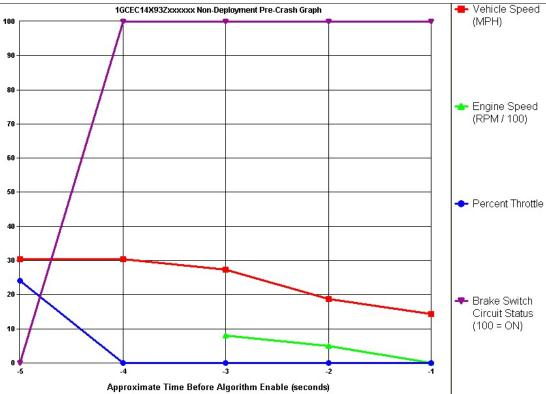
**Figure 26:** Case vehicle's pre-crash speed and brake switch circuit status showing that the vehicle's speed was recorded at 48 km.p.h. (30 m.p.h.) when the brake was activated approximately 4 seconds prior to algorithm enable.
