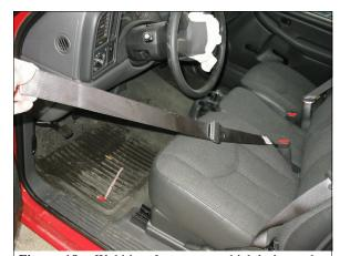
Figure 18: Webbing from case vehicle's lap only center seat belt showing blood on webbing (case photo #42)
