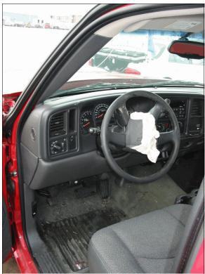
Figure 13: Case vehicle's driver seating area showing deployed driver air bag, greenhouse, left instrumental panel and knee bolster left of steering column, and toe pan areas (case photo #30)
