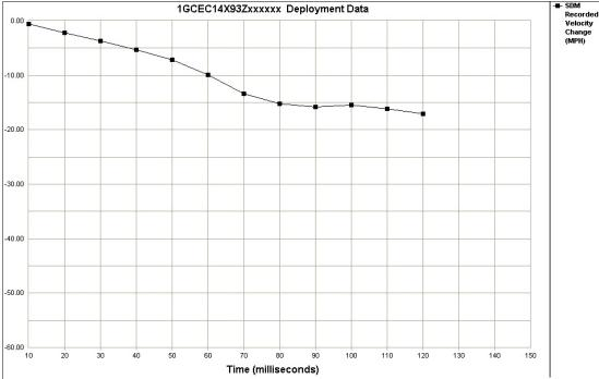
**Figure 24:** The case vehicle sustained a velocity change of approximately 27.4 km.p.h. (17.1 m.p.h.) during the first 120 milliseconds after the algorithm was enabled; maximum velocity change was recorded as 27.9 km.p.h. (17.4 m.p.h.) at 125 milliseconds.
