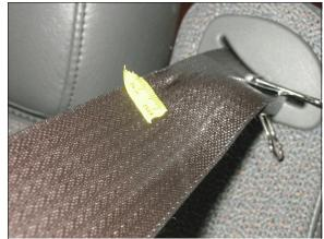
**Figure 21:** Close-up of loading evidence (i.e., "pinched" area) on webbing of case vehicle's integrated driver seat belt near retractor port (case photo #39)
