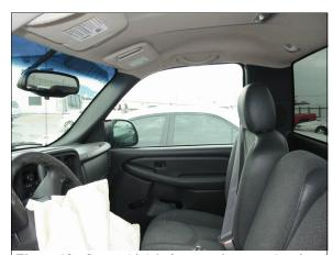
Figure 12: Case vehicle's front seating area showing deployed driver air bag and greenhouse area and rear view mirror above front center seat (case photo #28)
