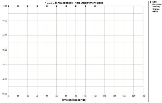
**Figure 27:** The case vehicle sustained a velocity change of approximately 0.0 km.p.h. (0.0 m.p.h.) during the first 100 milliseconds after the algorithm was enabled; maximum velocity change was recorded as 0.06 km.p.h. (0.04 m.p.h.) at 10 milliseconds
