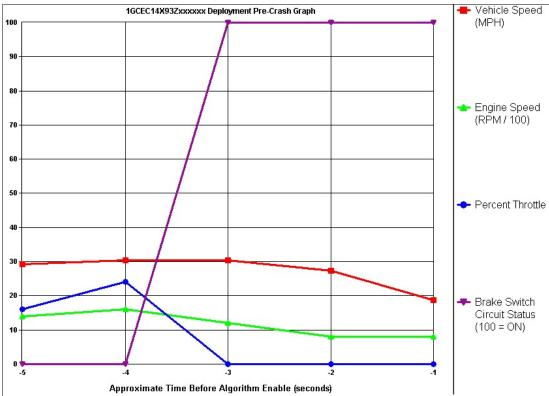
**Figure 23:** Case vehicle's pre-crash speed and brake switch circuit status showing that the vehicle's speed was recorded at 48 km.p.h. (30 m.p.h.) when the brake was activated approximately 3 seconds prior to algorithm enable.
