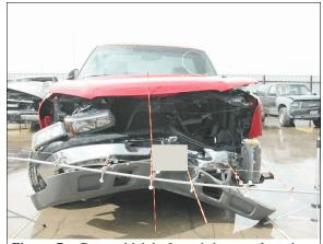
Figure 7: Case vehicle's frontal damage from impact with Ford; Note: contour gauge positioned at bumper level (case photo #16)
