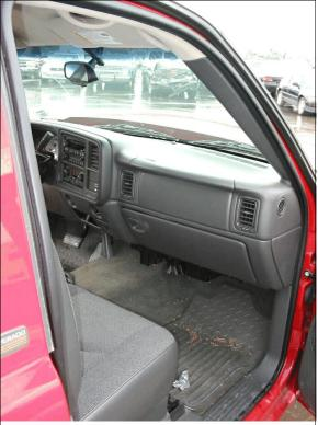
**Figure 14:** Case vehicle's front right seating area showing non-deployed front right passenger air bag, greenhouse, center and right instrument panel, and right toe pan areas (case photo #32)
