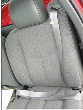
**Figure 20:** Elevated view of webbing from case vehicle's integrated driver seat belt showing loading evidence near retractor port (case photo #37)
