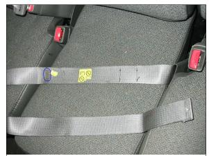
**Figure 19:** Overhead view of case vehicle's front center seat cushion and seat belt webbing; Note: blood (circled) on belt's webbing (case photo #45)
