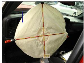
Figure 17: Case vehicle's deployed driver air bag showing possible blood evidence (arrow) on air bag's fabric near 4 o'clock area (case photo #33)
