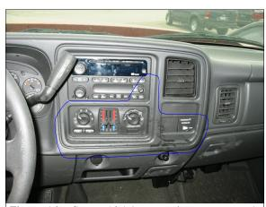
Figure 16: Case vehicle's center instrument panel area showing possible contact evidence; Note: splatters are not blood stains (case photo #40)
