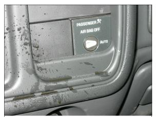
**Figure 9:** Close-up of case vehicle's front right passenger air bag switch located in lower right portion of center instrument panel; Note: switch located in "Auto" position (case photo #41)
