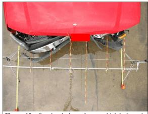
Figure 10: Overhead view of case vehicle's frontal damage showing contour gauge positioned at bumper level; Note: case vehicle was in counter-clockwise yaw at impact (case photo #27)
