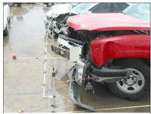
Figure 8: Reference line view of case vehicle's frontal damage viewed from left; Note: case vehicle's left front wheel is restricted by damage (case photo #19)
