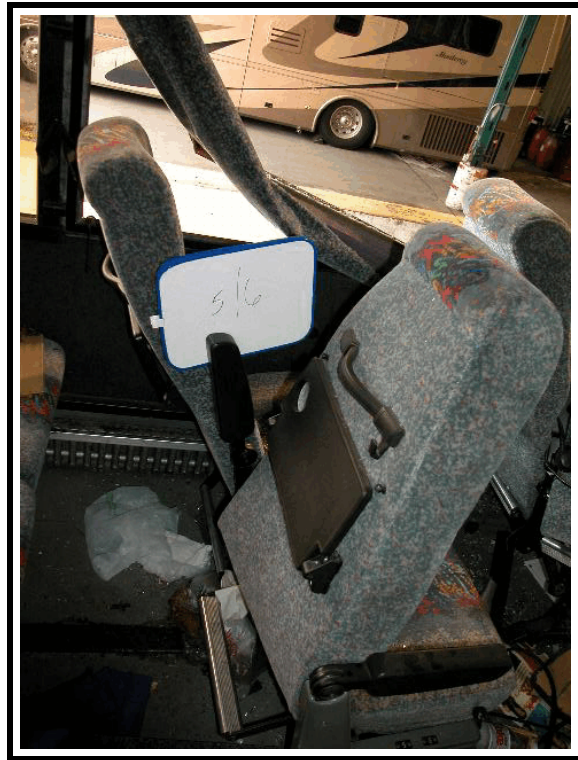
Figure 12. Example of seat back deformation. Bus row 2, aisle seat
