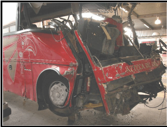
Figure 10. Front right, shows crushed entry way
