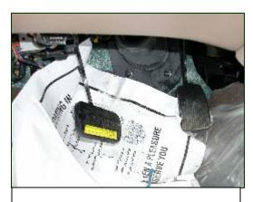
**Figure 8.** Deformed brake pedal from driver loading.
