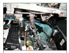
Figure 3. Adjustable pedal jackscrews.
