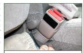
**Figure 10.** Fired driver's buckle pretensioner.
