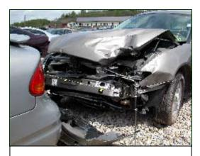
**Figure 5.** Frontal damage to the Ford Taurus.
