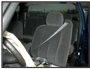
Figure 8. Integral driver's lap and shoulder belt
