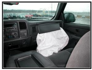
**Figure 10**. Deployed front right passenger air bag
