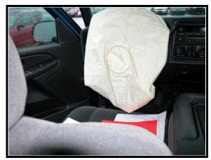
Figure 9. Deployed driver's air bag
