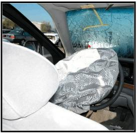
**Figure 8**. Driver's air bag / hand contact to windshield
