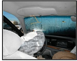
**Figure 6**. Contact damage to windshield and dislodged center mirror
