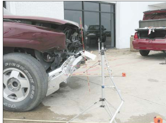
Figure 5: Right side view of crush to case vehicle's front bumper, each stripe on rods is 5 cm (2 in), the front baseline is set 17 cm (6.7 in) beyond the undeformed front bumper position
