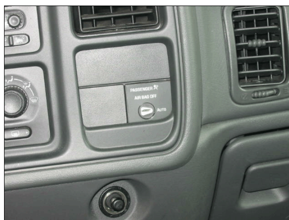
Figure 15: Front right passenger air bag suppression switch set to "AUTO" position
