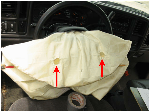
Figure 12: Driver's air bag vent ports
