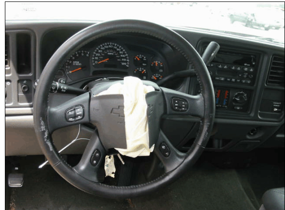
Figure 11: Driver air bag module cover flaps and the steering wheel
