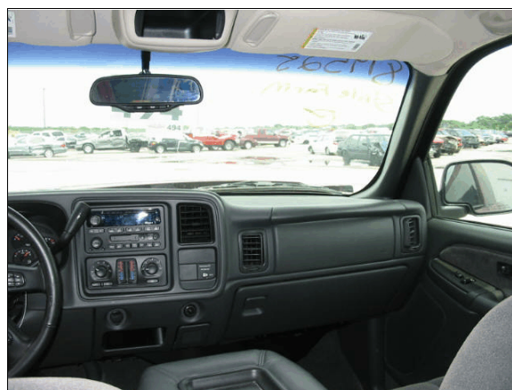
Figure 14: Overview of location of front right air bag in middle of instrument panel above glove box door
