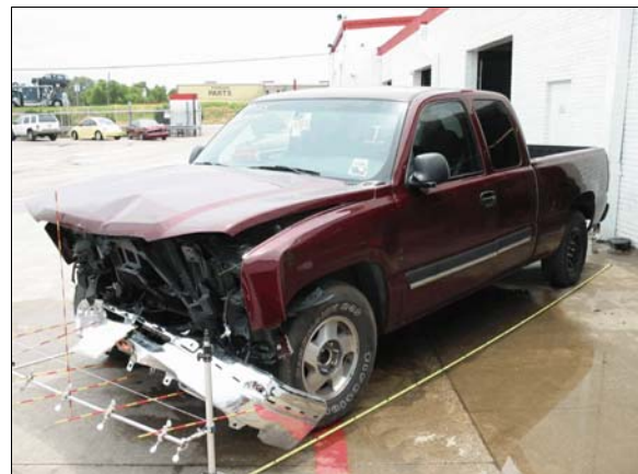
Figure 6: Overview of front and left side of case vehicle, each black mark on tape measure is 0.31 meter (1 foot)
