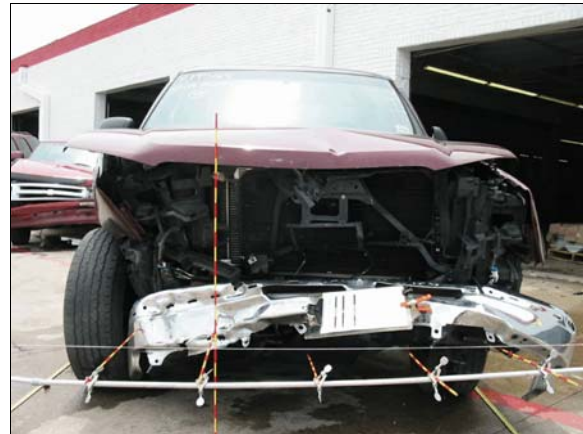
Figure 2: Front damage to case vehicle from impact with the median guardrail, each stripe on rod is 5 cm (2 in)
