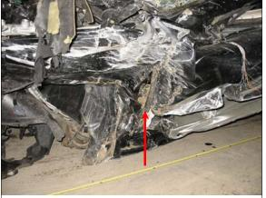
Figure 6: Dirt and grass jammed in left fender, left front door seam (arrow) and left front door (case photo #38)
