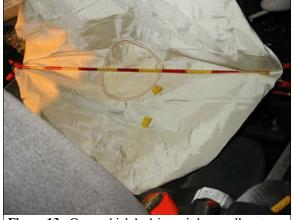
**Figure 13:** Case vehicle's driver air bag, yellow tape shows location of two small cuts in air bag (case photo #83)
