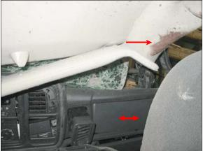
Figure 16: Passenger air bag located in middle of right instrument panel (double head arrow), arrow shows driver's head contact on right roof side rail (case photo #91)
