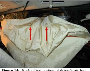
Figure 14: Back of top portion of driver's air bag, arrows show vent ports (case photo #88)
