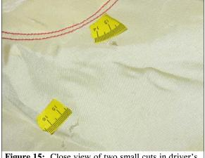
Figure 15: Close view of two small cuts in driver's air bag (case photo #84)
