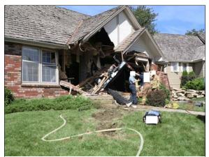
Figure 7: On-scene photo showing divot in ground from impact by case vehicle's left side and final rest of case vehicle in house (case photo #113)
