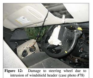
inches) of longitudinal intrusion of the steering assembly. The steering wheel was also broken due to impact by the intruding windshield header (**Figure 12**) and the steering column was compressed due to contact by the driver.
