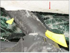
**Figure 18:** Close view of Figure 12 above showing hair deposit on center portion of windshield header, indicated by arrow (case photo #81)
