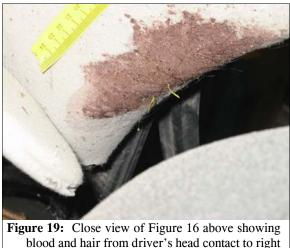
blood and hair from driver's head contact t roof side rail (case photo #92)
