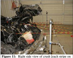
Figure 11: Right side view of crush [each stripe on rods is 5 cm (2 in)]to front of case vehicle (case photo #29)
