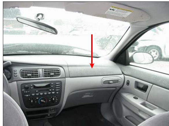
Figure 9: Case vehicle’s front right air bag located in middle of instrument panel above glove box door
