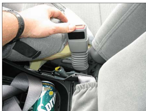
Figure 13: Front right seat belt buckle stalk is compressed indicating pretensioner activated
