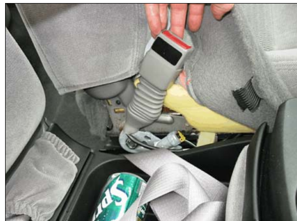
Figure 11: Driver's seat belt buckle stalk is compressed indicating pretensioner activated
