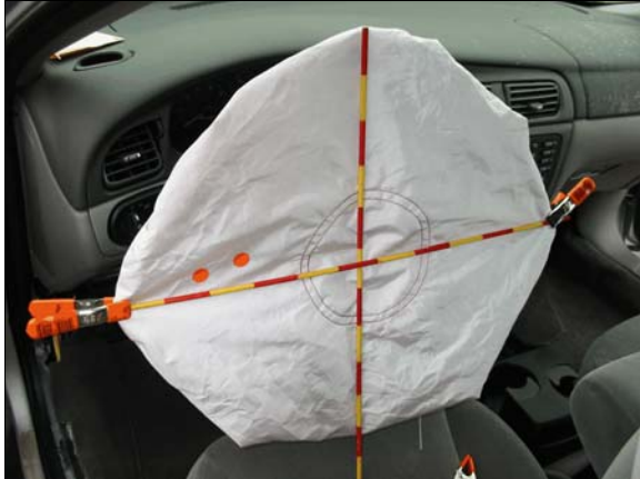
Figure 7: Case vehicle’s driver air bag, orange dots show small stain of unknown origin
