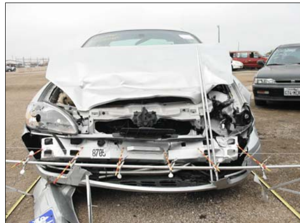
Figure 3: Damage to front of case vehicle due to impact with back of Chrysler, each stripe on rods is 5 cm (2 in)
