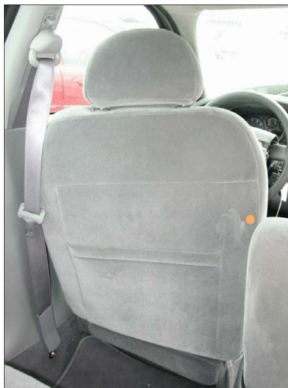
Figure 12: Back of driver's seat, orange dot shows occupant contact, seat back bent forward on right
