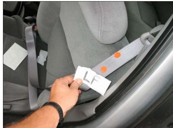
Figure 10: Case vehicle driver's seat belt, orange dots show small area of scuffing
