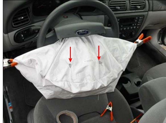
Figure 8: Back of top portion of case vehicle’s air bag, arrows show vent ports
