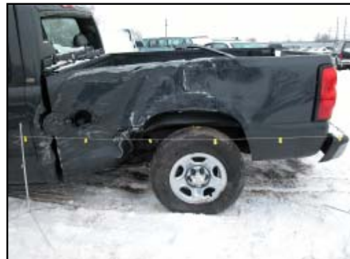
Figure 7. Left side damage from secondary impact with the Chevrolet Express.
