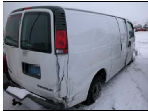
Figure 11. Damage from the secondary impact with the Silverado.
