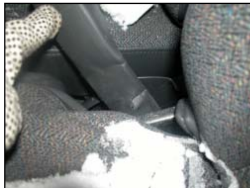
Figure 14. Damage to the driver's safety belt buckle sleeve.
