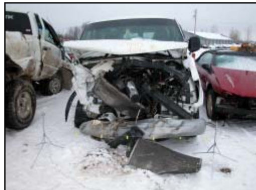
Figure 9. 2002 Chevrolet Express frontal damage.
