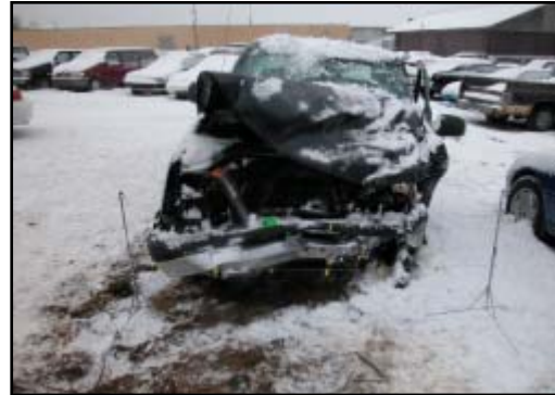
Figure 6. 2004 Chevrolet Silverado frontal damage.
