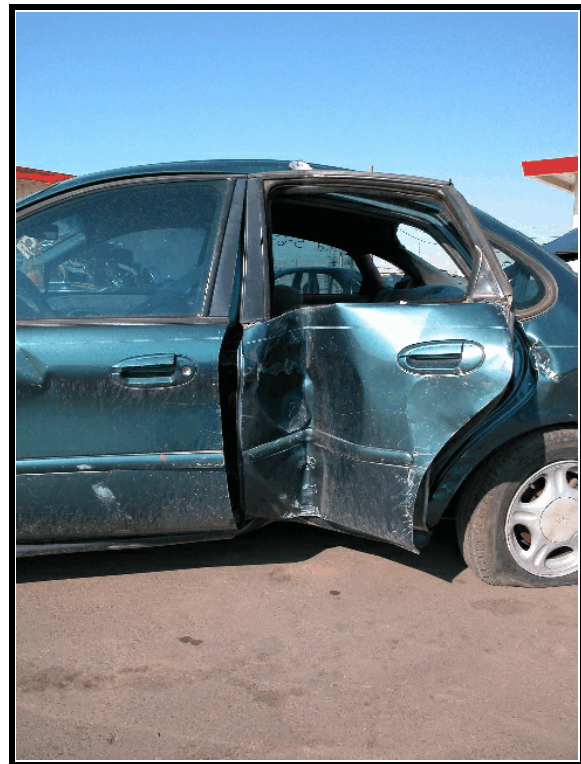
Figure 4. Pole impact to left rear door
