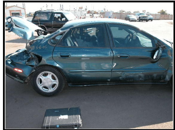
Figure 5. Right side rollover damage
