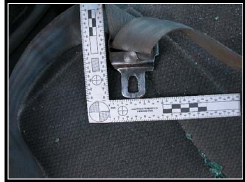
Figure 6. Lap portion of second row center seat belt.
