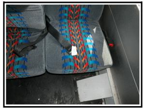
**Figure 19**. After-market lap belts - installed in all passenger positions
