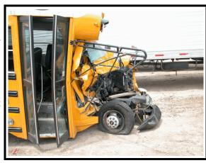
was a difference of greater than 13.0 cm (5.1 in) of crush at all of the C locations except C1. The averaged front crush was as follows: C1=37.0 cm (14.6 in), C2=39.5 cm (15.6 in), C3=54.0 cm (21.3 in), C4=79.5 cm (31.3 in), C5=83.5 cm (32.9 in), C6=98.0 cm (38.6 in).
