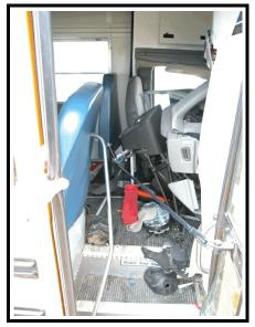
**Figure 16**. Instrument panel intrusion and damage to the right front door mechanics
