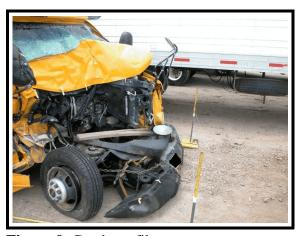
Figure 9. Crush profile
