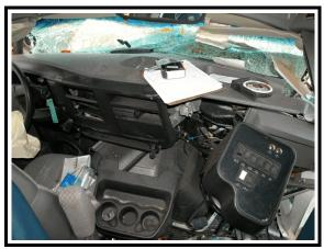
**Figure 14**. Instrument panel damage/intrusion
