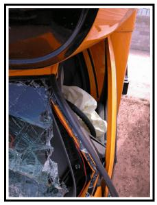
Figure 10. Damage to steering wheel/column and windshield integrity loss
