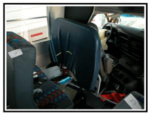
**Figure 25**. Padded divider separating driver and second row/left passengers
