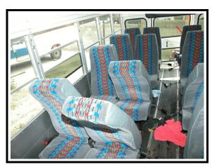
**Figure 18**. Passenger seat damage - right side
