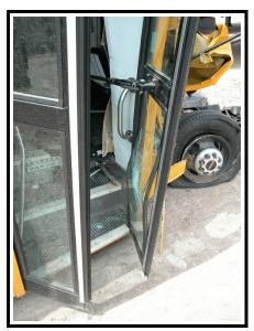
**Figure 11**. Damaged front entrance door
