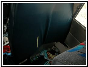
Figure 26. Padded divider separating second row/right seats from front entrance
