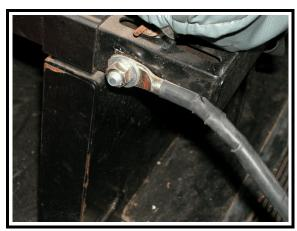
**Figure 22**. Closer view - After market seat belt buckle attachment point
