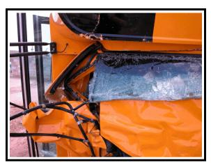
**Figure 12**. Windshield integrity loss - right side
